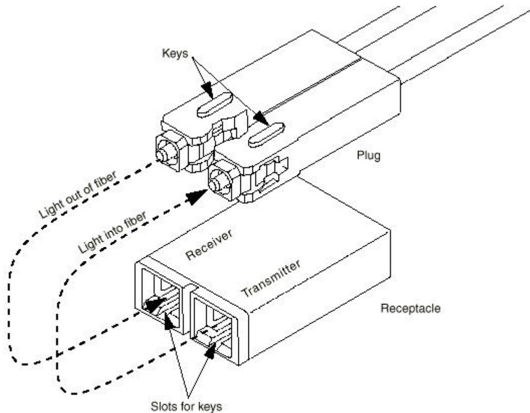
NOTE—Connector keys are used for transmit/receive polarity only. The connector keys do not differentiate between single-mode and multimode connectors.
