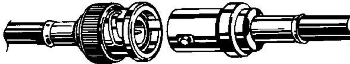
Figure 9.1–BNC connectors (10BASE2)
