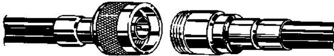
Figure 9.5–N series coax connectors (10BASE5)
