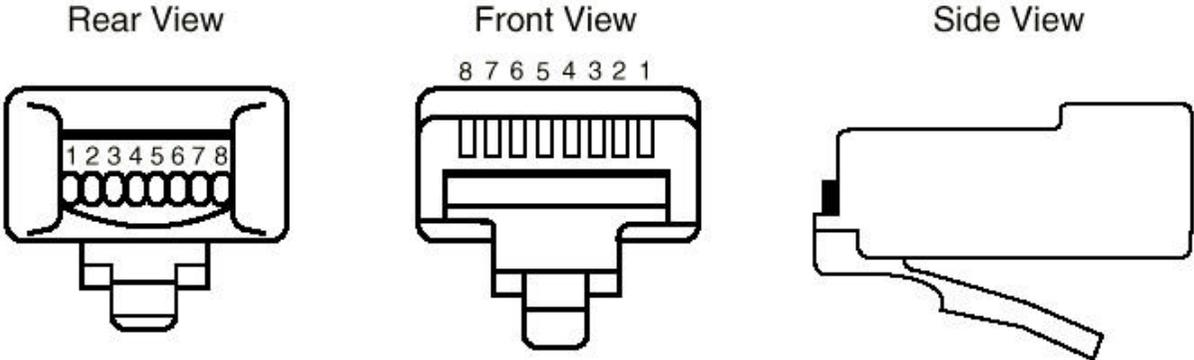
Figure 9.7–RJ-45 (8 pin) modular plug
