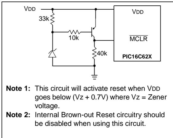
**FIGURE 9-14: EXTERNAL BROWN-OUT PROTECTION CIRCUIT 2**
