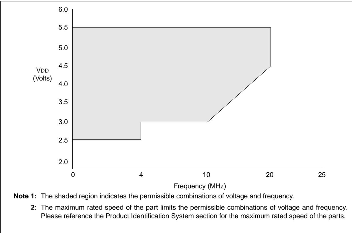
**FIGURE 12-7: PIC16CR62XA VOLTAGE-FREQUENCY GRAPH,  $-40^{\circ}\text{C} \leq T_A \leq 0^{\circ}\text{C}$ ,  $+70^{\circ}\text{C} \leq T_A \leq +125^{\circ}\text{C}$**
