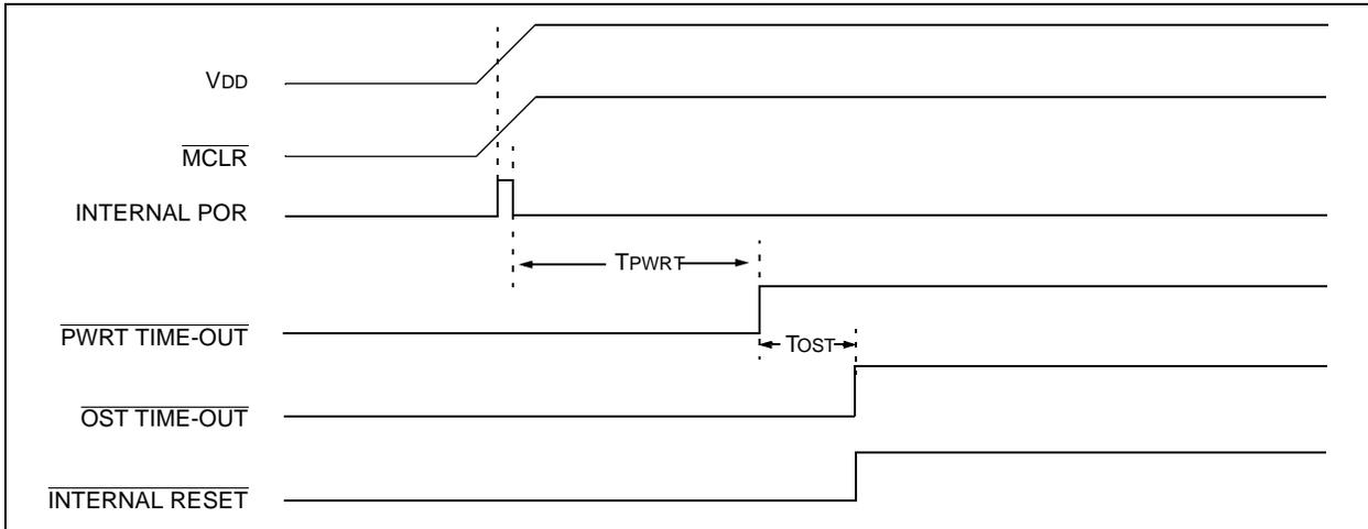
**FIGURE 9-12: EXTERNAL POWER-ON RESET CIRCUIT (FOR SLOW V<sub>DD</sub> POWER-UP)**
