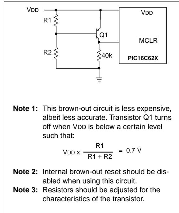
**FIGURE 9-15: EXTERNAL BROWN-OUT PROTECTION CIRCUIT 3**
